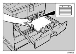
While pressing the release lever, push in the side and end fences until they are flush against the paper's edges.
